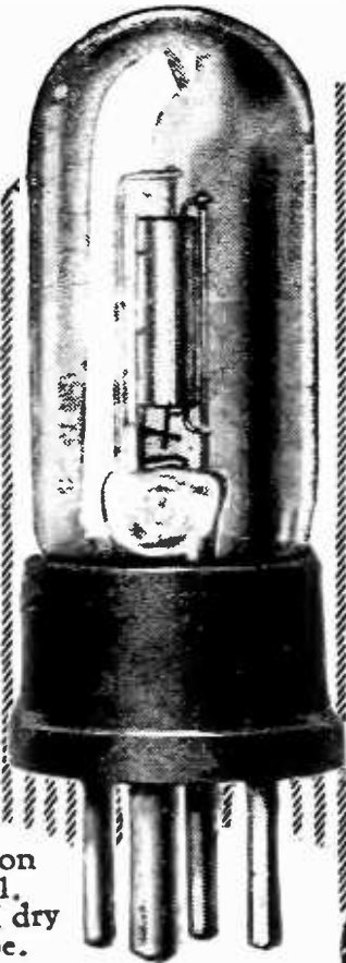
Radiotron WD-12. The standard base dry cell tube.
